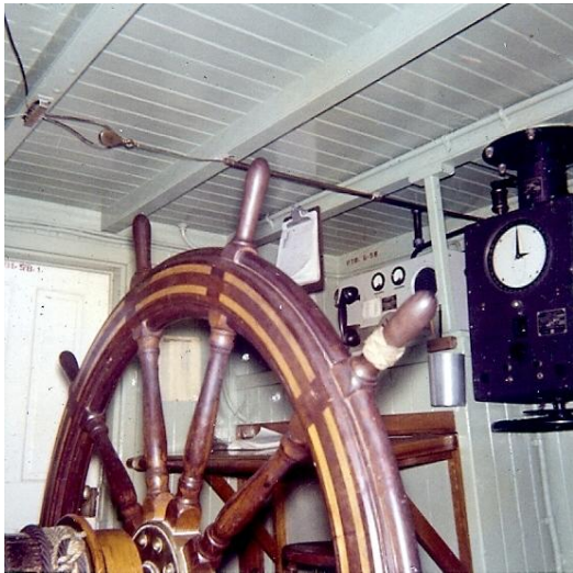
Wheel House with Radio & Log Station. Note, tongue & groove planking
